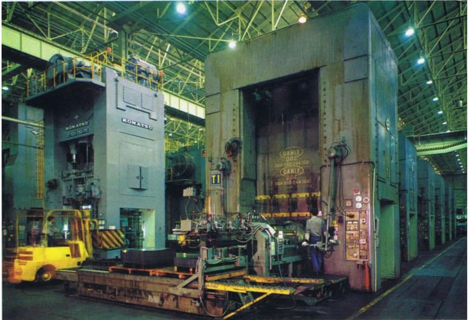
Danly QDC (Quick Change Die) machine at Toyota — image courtesy of Art Smalley
